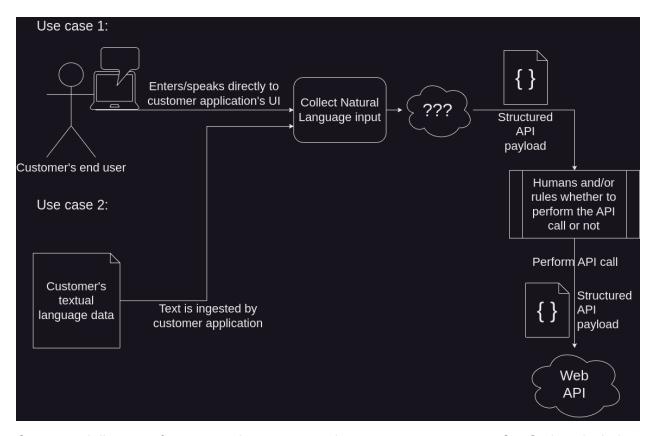
Conceptual diagram of two example use cases where a customer can use CueCode to include validation of generated API payloads.
