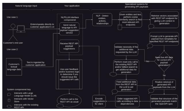
Current process flowchart for engineering REST API generation with OpenAPI specifications, showing the two example customer use cases from other slides. Major system components involved at each process step are labeled with icons.
